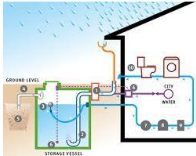
Fig. 10. Schematic Diagram showing how captured rainwater can be used in homes. Source: starkenenvironment.com, 2012.
