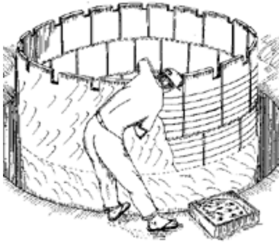
Fig. 16. A RWH tank made of pre-cast concrete plates. Source: UNEP, 2009
