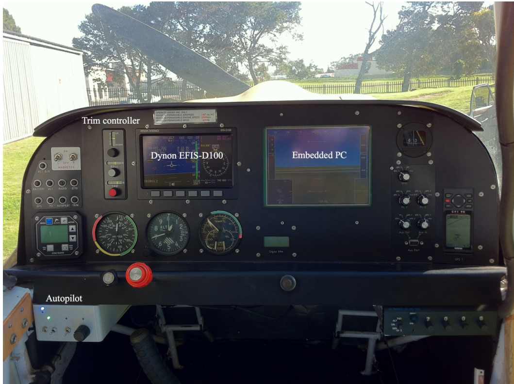
Figure 3.13: The instrument panel of the test aircraft, showing the Dynon EFIS-D100, the embedded PC, the trim controller and the autopilot.
