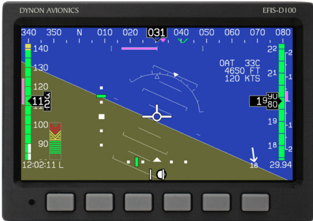
Figure 3.11: The presentation of air data on the Dynon EFIS-D100. [2]
