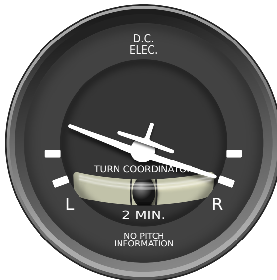
Figure 2.7: Illustration of a turn coordinator, an instrument that shows the rate of change of heading, and indicates an imbalance in the controls (Copyright © Oona Räsänen, used with permission).
