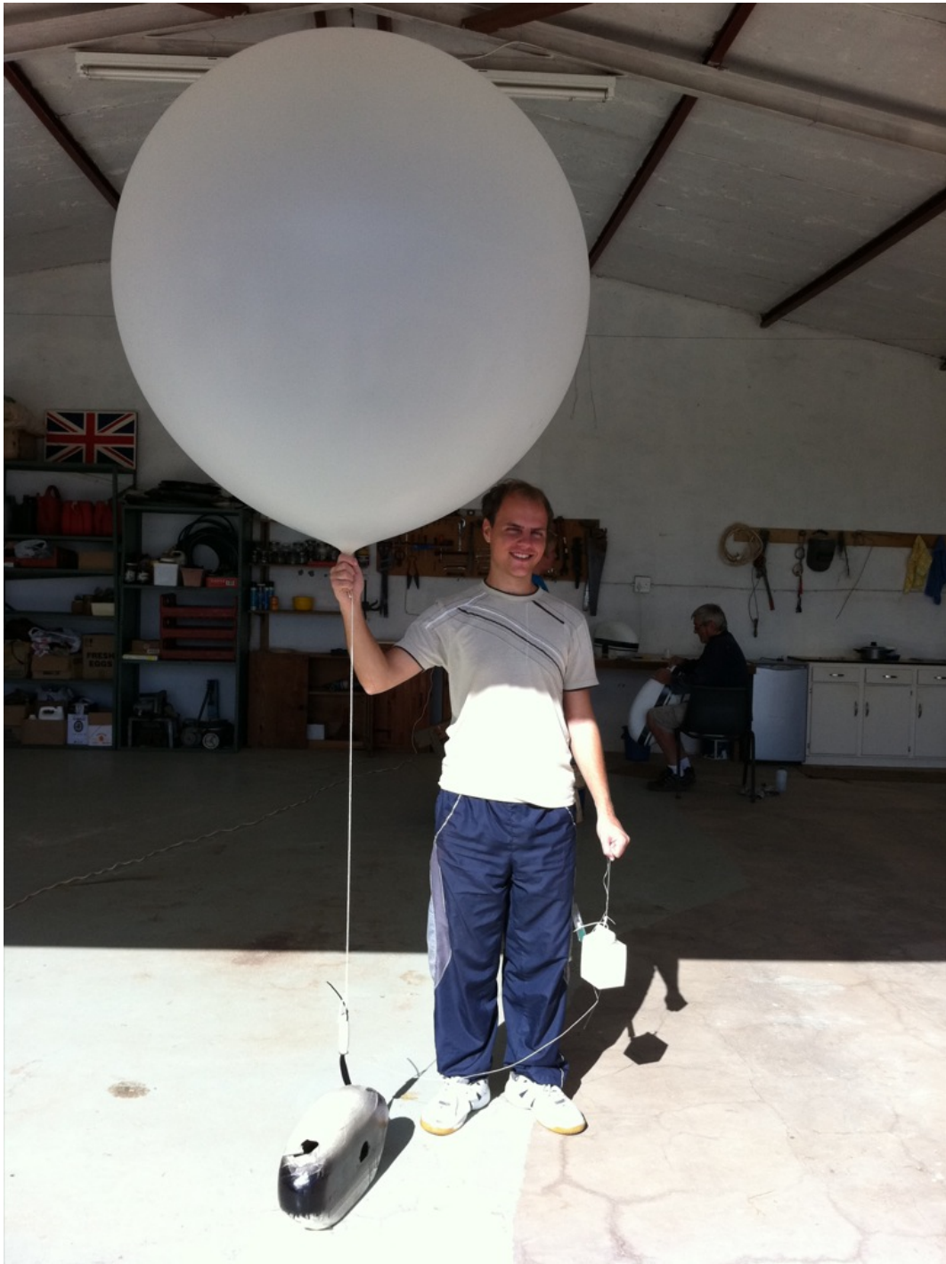
Figure 3.14: A weather balloon with radiosonde attached, prior to launch
