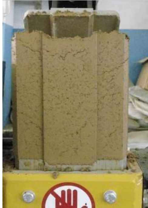
Figure 4: Block mixture too wet, horizontal cracks formed, block sticks to rammer
