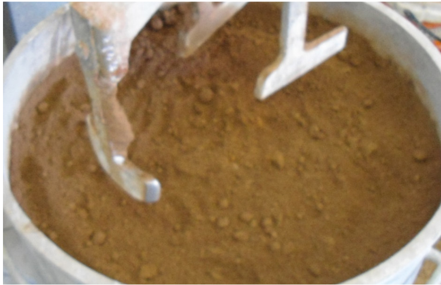
Figure 13: Example of soil-cement 'balling' effect when mixed with a pan mixer
