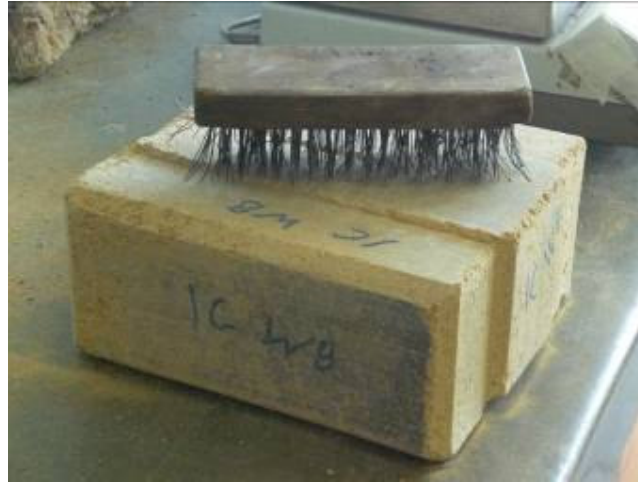
Figure 30: Oven dried block and wire bristle brush
