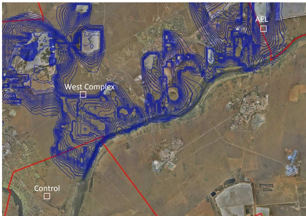
Figure 1.4. The locations of the three study sites (white blocks) and the associated contamination plumes (blue lines) (GCS, 2007).
