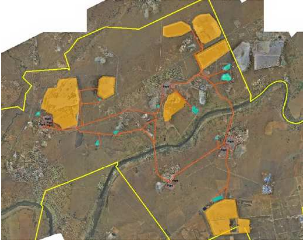
Figure 1.1. The Tailing Storage Facilities (yellow blocks) and associated tailing pipes (red lines) found in the AngloGold Ashanti Vaal river region (AngloGold Ashanti, 2007a).
