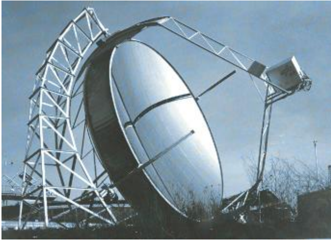
Figure 10: Solar Dish design [34]
