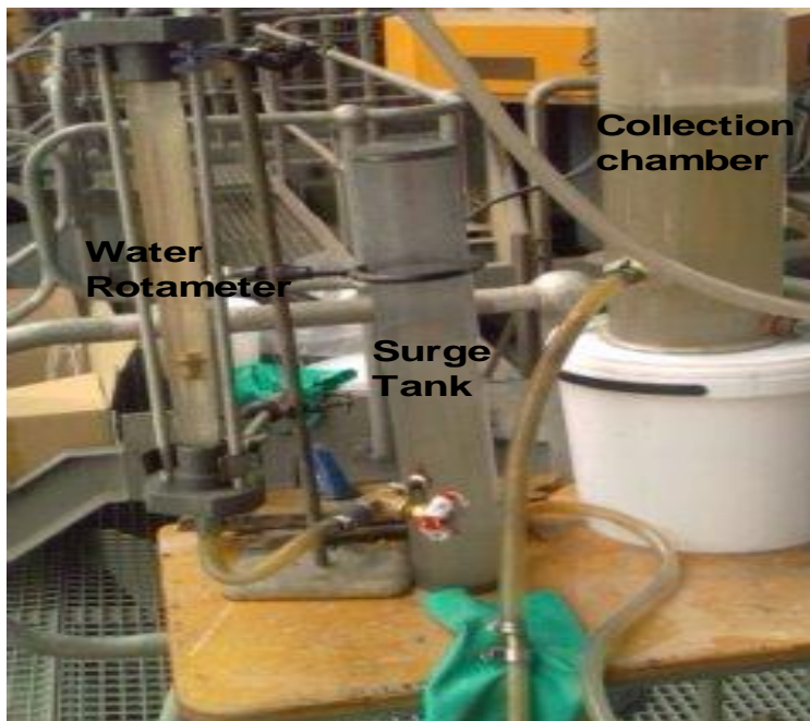
Figure 3.11: Photograph showing the collection chamber, surge tank and water rotameter during bubble load measurement.
