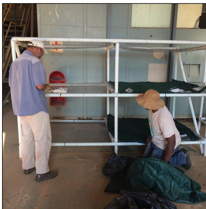
Figure 3.8. Chicken mesh drying shelves for drying bags of S. lancea leaves.
