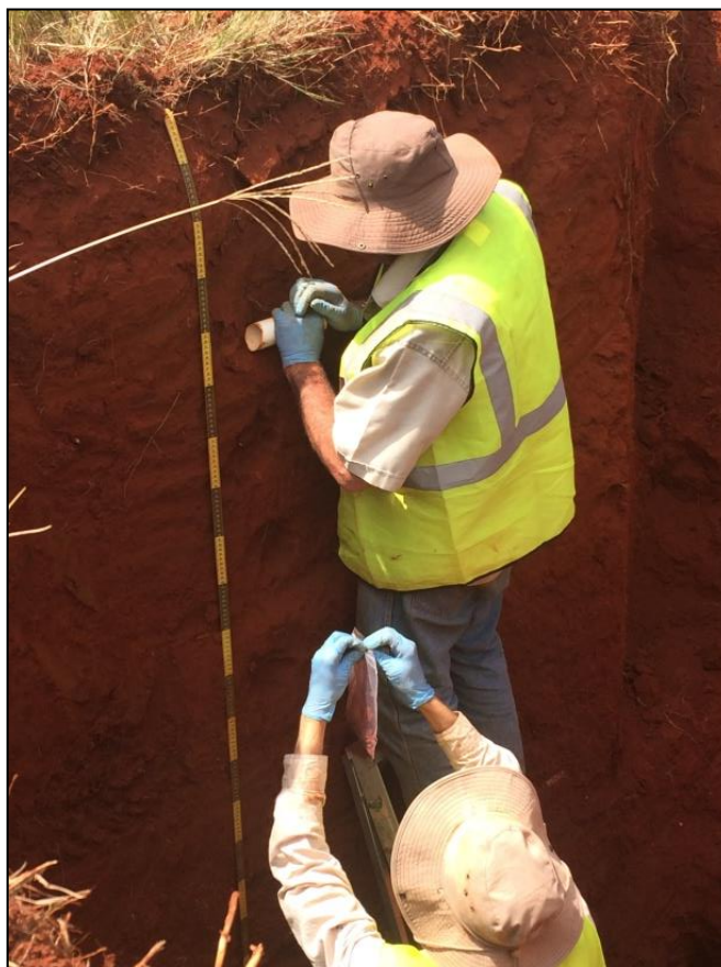
Figure 3.10. Soil pit sampling in progress using the specially cut PCV pipe.
