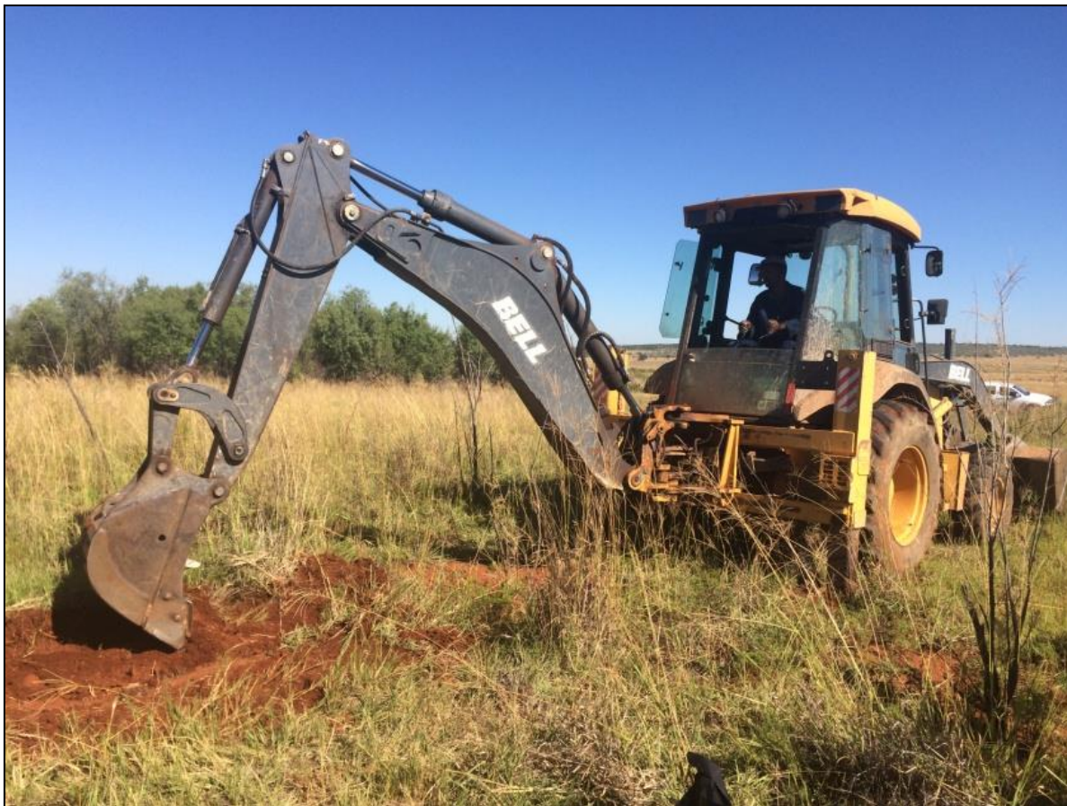
Figure 3.3. TLB breaking ground on the first soil pit at Redsoils, West Wits site.
