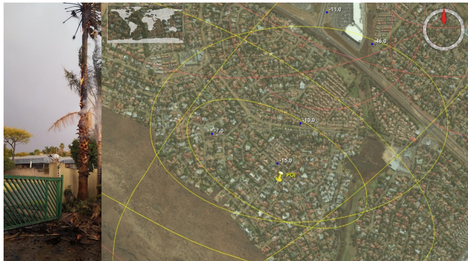
Figure 1.3: Example of burning damage with location map data of possible sources for lightning attachment
