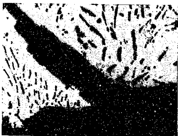
Figure 4.3 Graphite Flakes in Iron (x 400)
