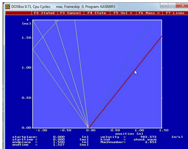
Figure 80: Case F Shock wave diagram
