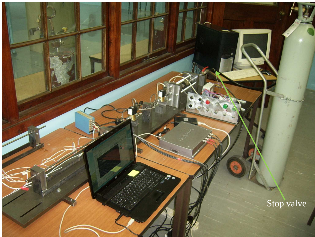
Figure 39: Shock tube rig components assembly
