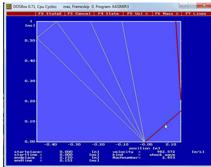
Figure 75: Case A Shock wave diagram
